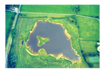
It was constructed out of the natural clay with White Horse Contractors' earth moving equipment, utilising a cut-and-fill operation and building up levels on two sides of the field.
